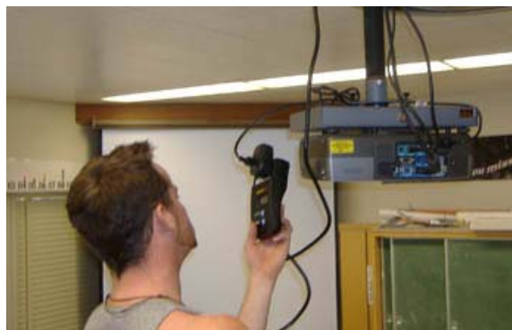
Scott Willingham, one of over a dozen volunteer auditors, measures a phantom load of a projector in Harry Griffith Hall.
