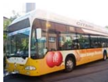
Stuttgart's fuel cell bus parked outside of the Whirlpool factory.
